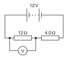
There is a voltmeter connected across the  $12\Omega$  resistor.
